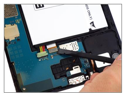
Use the flat end of a spudger to lift up and disconnect the LCD screen press-fit connector.
