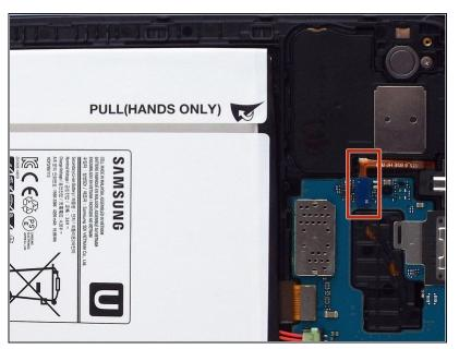
Use the flat end of a spudger to lift up and disconnect the 3.5mm headset jack press-fit connector.
