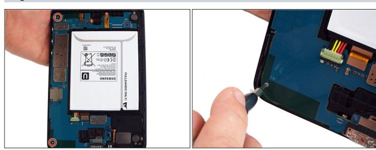
Use a PH000 screwdriver to remove the two 3 mm screws on the left side of the motherboard.
