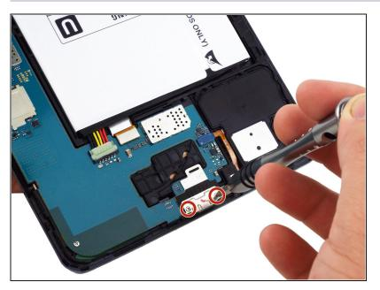
Use a PH000 screwdriver to remove the two 3 mm screws that connect the USB port shield to the midframe.
