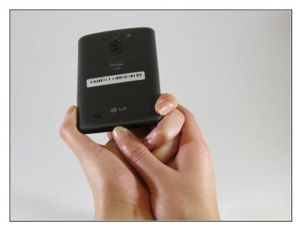
Remove the back cover by gently prying open the case of the device from the charging port.
