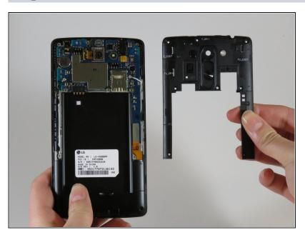
Use a plastic spudger, or finger nail, to lift up the hard shell on the top of the phone.
