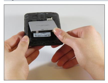
Lift the battery out of its place by prying up from the small notch at the base of the battery.
