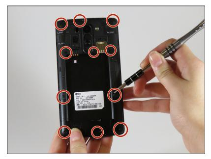
Using a Phillips #000 screwdriver, remove the eleven 3.0 mm screws around the perimeter of the phone.
