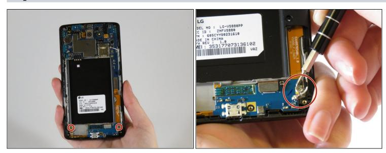
• Using a Phillips #000 screwdriver, remove the two screws from the device.
