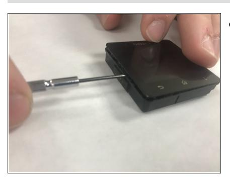
Use a plastic opening tool to carefully pry the LCD screen from the watch housing.
