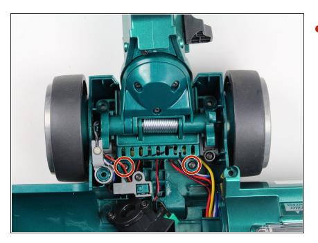
Remove two 14mm screws by rotating counter-clockwise with a T15 Torx screwdriver.
