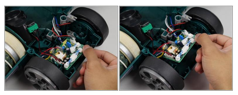
• Lift the motherboard out of its compartment.
