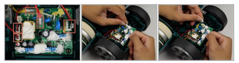
Locate and remove these connections by pulling the plugs out of the sockets.
