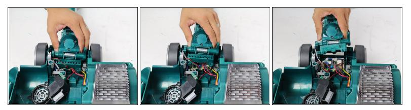
• Lift and gently remove the hinge compartment covering the motherboard.
