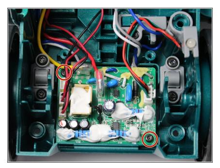
Remove the two 10mm screws by rotating counter-clockwise with a T10 Torx screwdriver
