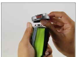
Remove the cap by pushing the "pull" tab.
