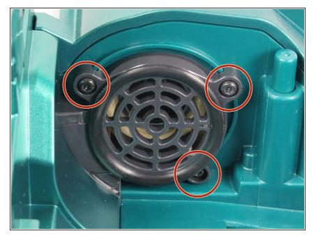
Remove three 10mm screws by rotating counter-clockwise with a T15 Torx screwdriver.
