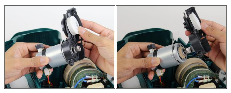
• Remove the belt-assembly unit by pulling the belt-assembly unit away from the motor.
