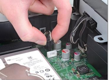
Unplug the bundled cable connector connecting the hard drive to the motherboard by pulling directly upward.
