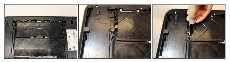
Remove the left spring by grabbing the rubber tips connected to the spring and lifting up.
