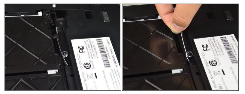
• Remove the right spring by grabbing the rubber tips connected to the spring and lifting up.
