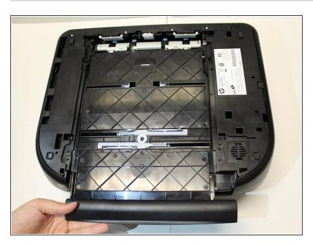
Remove the paper tray by pulling the tray away from the printer.
