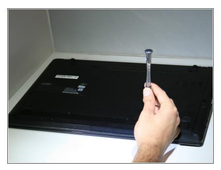
Unscrew the two screws using a Phillips #0 screwdriver.
