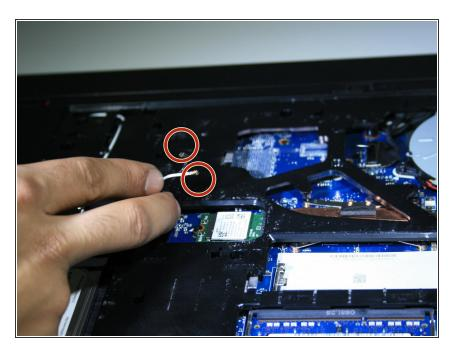
Unplug the two wires that are on the Wi-Fi PCI card (white & black).
