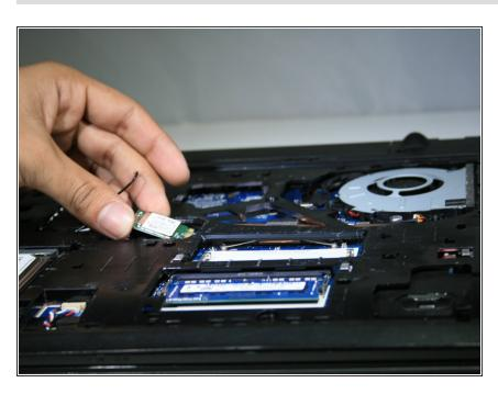
Remove the Wi-Fi PCI card from the device.
