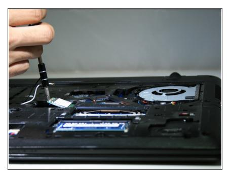
Unscrew the single screw in front of the Wi-Fi PCI card using the Phillips #0 screwdriver.
