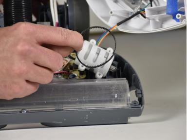
Remove the belt by sliding it off the end of the motor.
