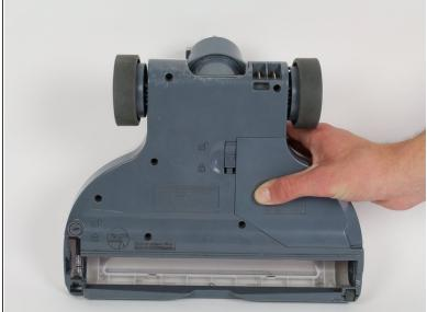
Slide the latch next to the panel upwards into the unlocked position.
