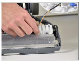
Remove the 12.2 mm Phillips #1 screws holding the motor in place and remove the motor by pulling directly upwards.
