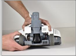
Remove the bottom panel from the vacuum by pressing to release the latches at the front and pulling the bottom panel away from the vacuum.
