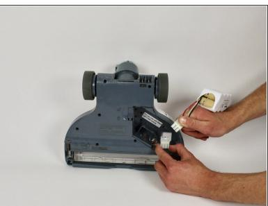
Disconnect the battery from the vacuum by pinching the white latch and pulling the two pieces apart.
