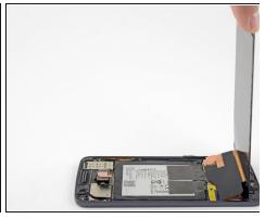
• Lift the earpiece end of the display up to provide access to the display cables.
