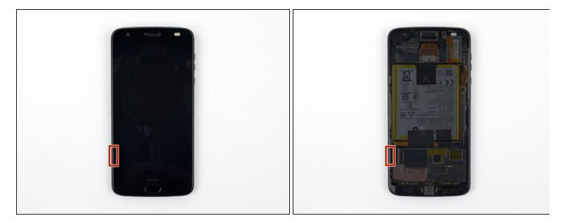
When separating the left side of the screen assembly, take care to not snag the display cable located on the left edge near the bottom of the display.
