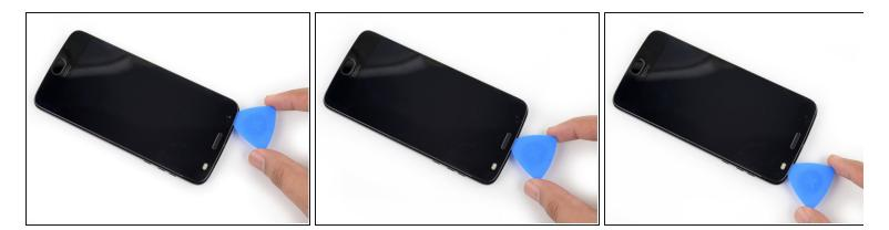
Slide your tool around the top edge of the screen assembly and slice all along it to slice through its adhesive.
