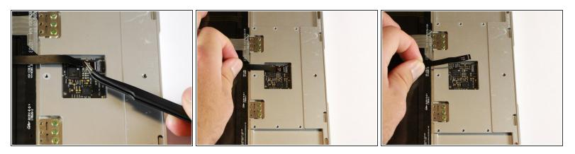
Gently pull out the ribbon connector either by using tweezers or your fingers to pull the cord out and up.
