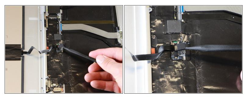
• Remove the small, black casing by using the spudger to lift it up from its place.
