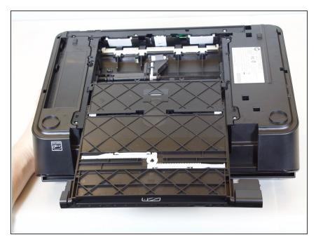
Pull the paper tray out until it hits the stops on either side of the tray.
