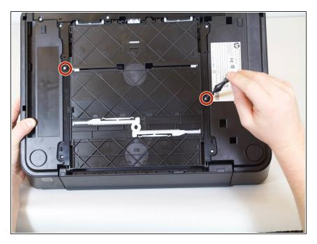
Use the T-10 screwdriver to remove the two 11-mm screws.
