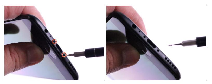
Remove the two 1mm Torx #2 screws at the bottom of the phone by rotating the screwdriver counter-clockwise.
