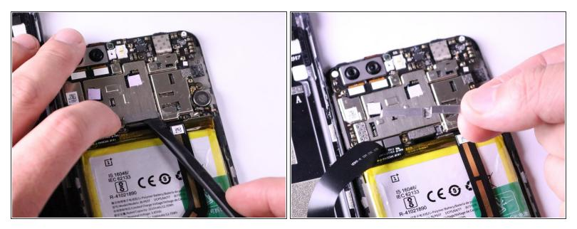
• Carefully pop out the metal connector cap with the nylon spudger and remove it by pulling up.
