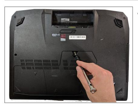
Unscrew the 5.2mm screw underneath the flap.
