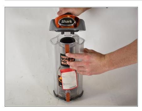
A dust filter is located within the dust cup. To access it, open the dust cup by pressing the orange tab on the front and pulling up on the handle.
