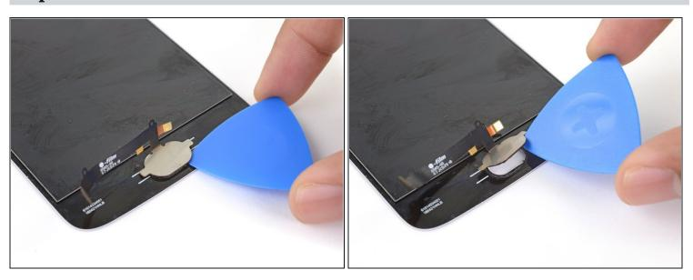
Carefully pry off the fingerprint sensor by lifting it with the edge of an opening pick.
