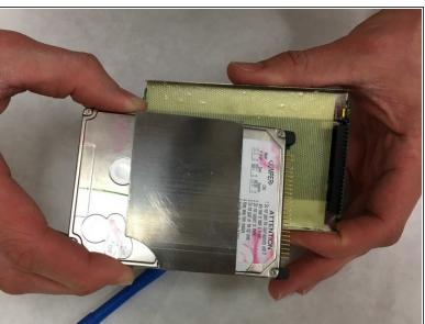
Lift the hard drive out of its casing with the help of a plastic opening tool and slide it out. This will
