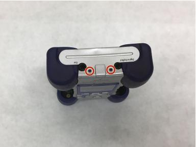
Remove the 2 screws on the top and the 2 screws on the bottom of the device using a Phillips #0 screwdriver.
