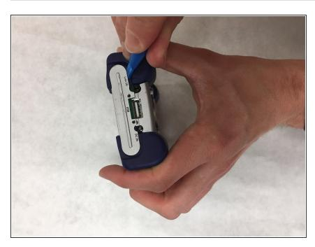
Remove the outer metal casing of the device by popping it off with a plastic opening tool.
