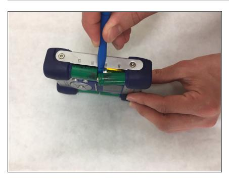
Remove the batteries (may require a plastic opening tool or spudger to pop the batteries out).
