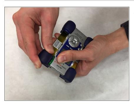
Remove the rubber bumpers on all four corners of the device.
