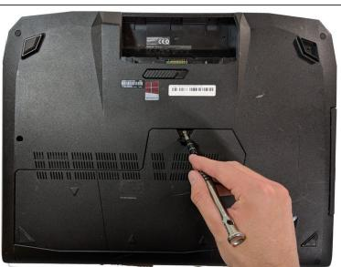
Open flap in center and underneath you will find a screw, remove the 5.2mm screw with a Phillips #0 screwdriver.
