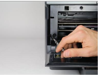
Remove the two 13mm screws with a T9-TORX screwdriver by turning counter-clockwise (left).
