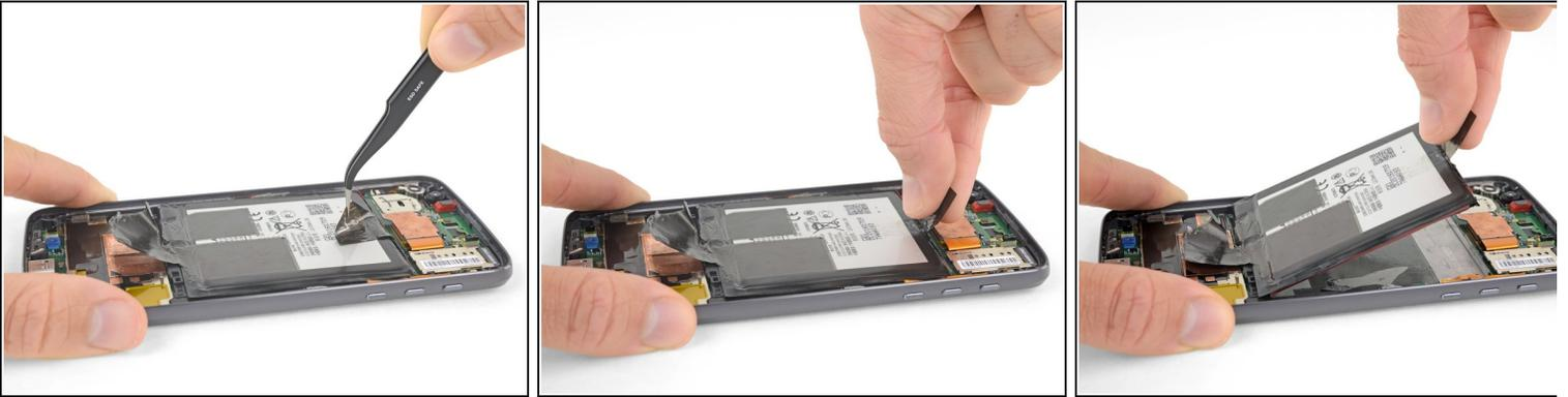
**⚠** In the following steps you will only lift the battery, **do not completely remove it**—it's still connected to the motherboard.
