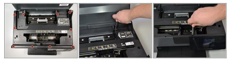
Use a T9 torx screwdriver to remove a total of ten (10) 12mm screws from the main cover by turning the screwdriver counterclockwise.
