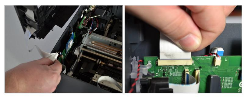
Grab the base of the white ribbon cable connecting the cover to the base of the printer and pull it out.
