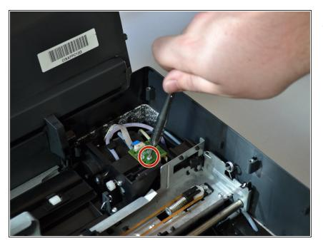
Twist the screwdriver counterclockwise to remove the T9 screw on the sensor chip.
