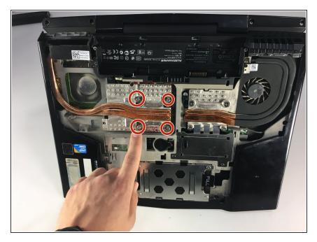
Remove the heat sink by loosening the 4 screws with a Phillips #0 screwdriver.
