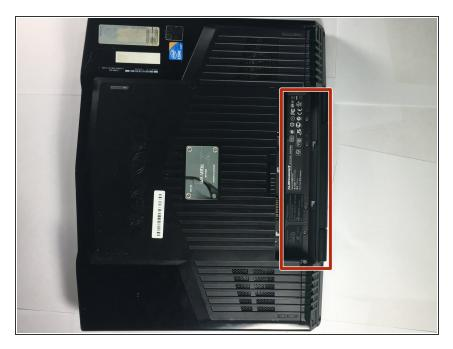
Release the battery latch and flip the battery out.
