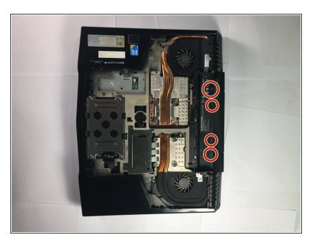
Remove the four 4mm screws with the Phillips #1 screwdriver.
