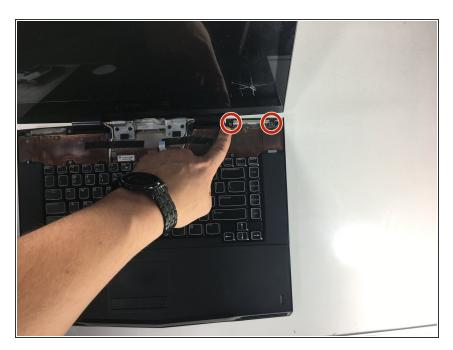
Remove the two 4mm screws with a Phillips #1 screwdriver.
