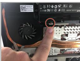
• Use a Phillips #0 screwdriver to remove the two 3mm screws holding the fan in place, then unclip the electrical connection using tweezers.
