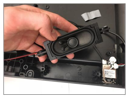
Pull the speaker out of its casing, and repeat for the process for the other speaker.
