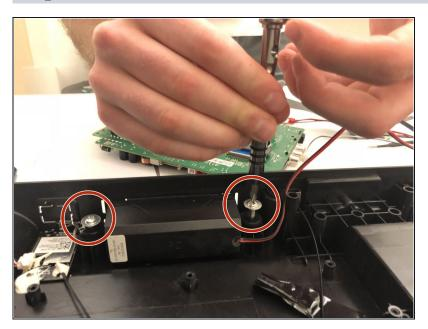
Remove screws on both sides holding the speaker in place.
