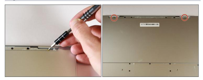
• Remove the two yellow 2.0mm screws by using a T3 Torx screwdriver.
