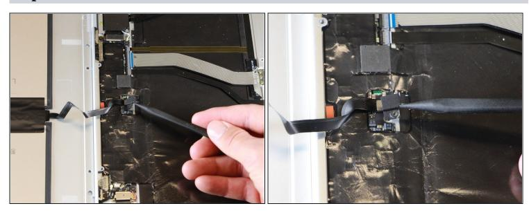
• Remove the small, black casing by using the spudger to lift it up from its place.
