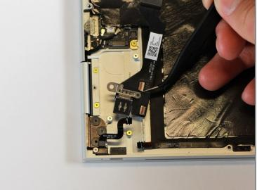
• Remove the right charging port by picking it up with the <u>tweezers</u> and lifting it from the computer.
