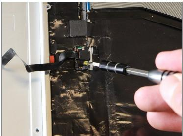
• Remove the yellow 2.0mm screw from the middle of the panel by using the T3 Torx screwdriver to turn the screw counterclockwise.
