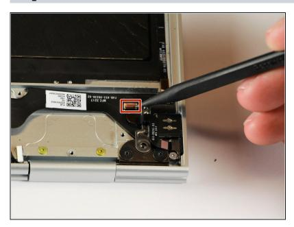
Remove the small, red component by lifting it up with the spudger.
