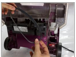
Remove the belt that's to the right of where the brush roll was by pulling the bottom off of the pin.
