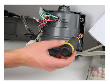
Unscrew two screws with Phillips #2 screwdriver.
