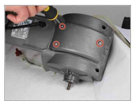
Flip vacuum over and unscrew three screws with a Phillips #2 screwdriver.
