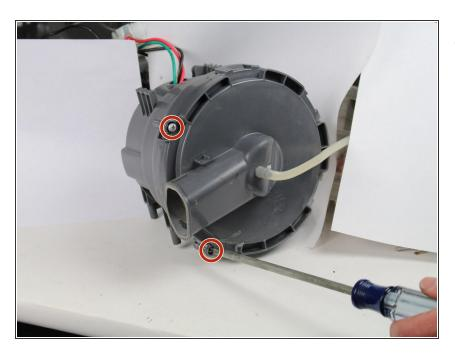
Detach motor and unscrew two screws with a Phillips #2 screwdriver.
