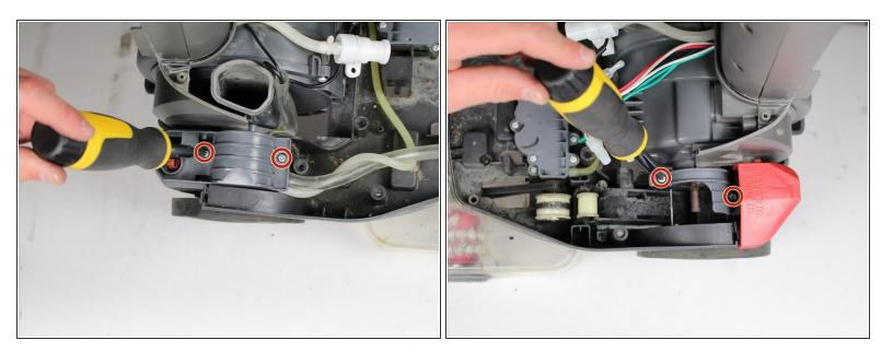
• Unscrew four screws using a Phillips 2 screwdriver.
