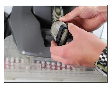
Grab the attachment at tip of the hose and unscrew it. Pull outwards on the hose until completely removed.
