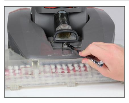
Unscrew the Phillips #2 screw at the bottom of the hose.
