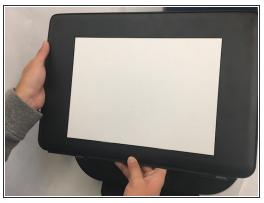
• Take the cover off by popping the cover's hinges from the rest of the printer.
