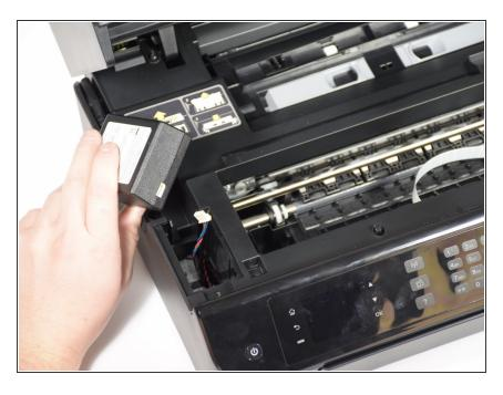
Remove final cable from power supply.
