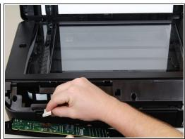
Gently remove the No-Fuss ribbon cable from the front panel.
