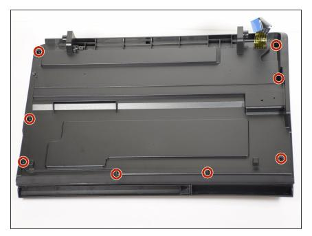
Remove eight T10 1mm screws from the top hood of the printer.
