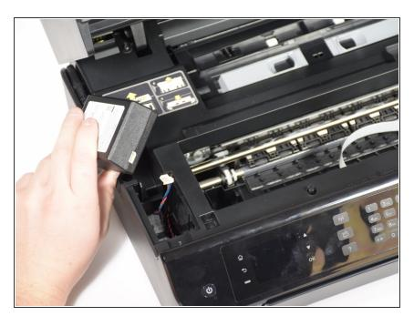
Remove final cable from power supply.
