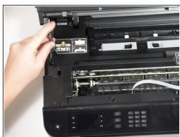
Remove the two T10 11mm screws.
