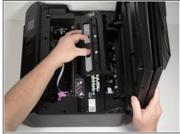
Remove the paper feed rollers by using your fingers to pinch the indentations together while pulling up.
