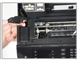
Remove the panels covering the power brick and cord.
