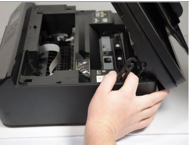
Remove the clip that keeps the printer lid from opening all the way with your hands by pulling away from the post on the lid.
