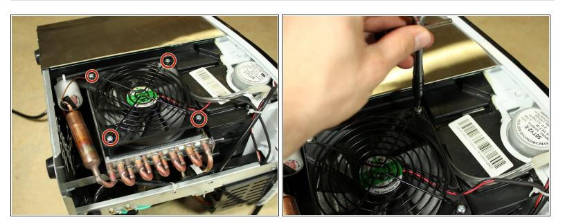
Locate the fan on the side of the Ice maker and undo the 4 screws holding it in place.
