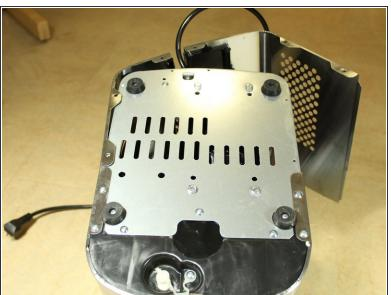
• Undo the 6 Screws found on the bottom edge holding the rear casing on.
