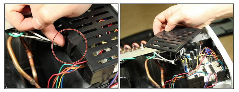
Remove the cover from the circuit board by pressing against the lever to the side. A pry tool may be needed.
