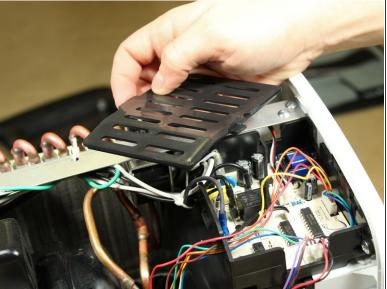
Remove the plastic cover over the circuit board by pressing the lever on the side. A pry tool may be required.
