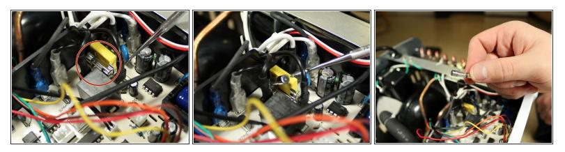
Remove the fuse with a plastic pry tool.
