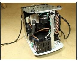
Remove the 6 screws along the bottom of the rear casing.
