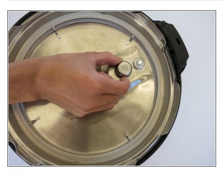
• Pinch the anti-block shield and twist counterclockwise while pulling up and out from the lid.
