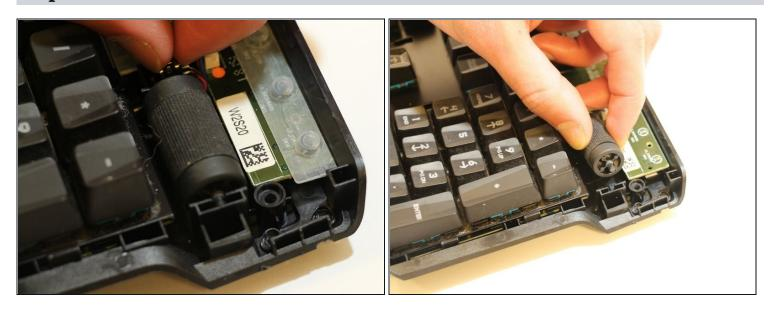
• Using your fingers, gently remove the volume control wheel from the device.
