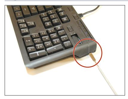
Push the metal spudger underneath the two layers of the keyboard. Using your hand to add pressure, push it downward revolving it to open.
