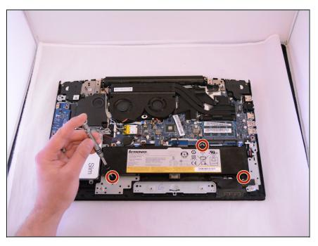
Use the Phillips #0 screwdriver to unscrew the three screws holding the battery.
