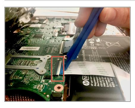
Remove the thick white ribbon cable covering the battery using the plastic opening tool by prying up the latches attaching each end.
