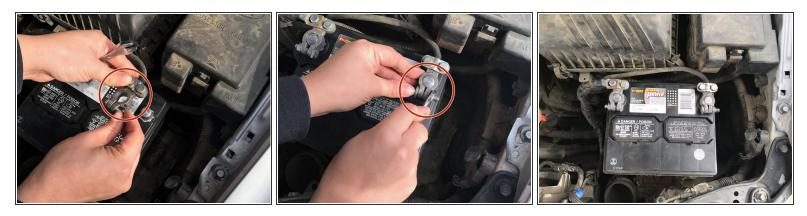
Then, attach the negative (red arrow) cable to the battery by screwing on the nut and bolt with the wench.
