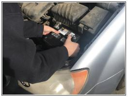
Place the new battery in the base where the battery goes.
