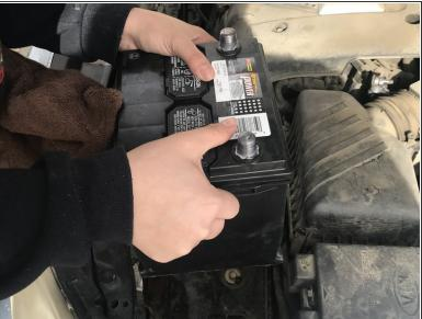
Take the battery out, lifting the battery.
