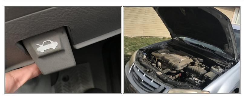
• Locate the hood release lever near the lower left side of the steering wheel. Pop the hood by lifting up on the release lever.
