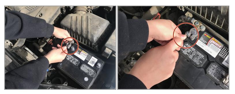
Attach the positive (red cirlce) cable to the battery by screwing on the nut and bolt with the wrench.
