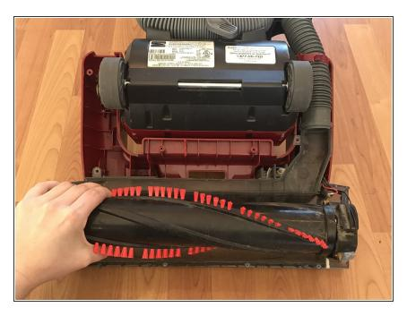
• Remove the brush roll completely by pulling it out.
