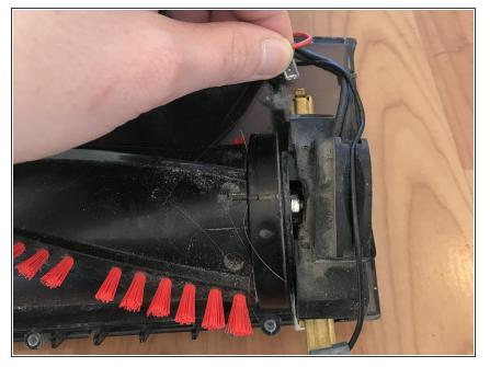
• Remove the positive motor terminal that is located on the upper right corner of the brush roll.
