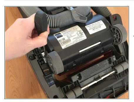
Using a Phillips 2 screwdriver, remove the 10-32 x 1/2" screw from the pedal to make room for the removal around the wheel.
