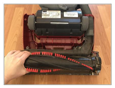
• Lift the brush roll out of the vacuum by pulling it up.
