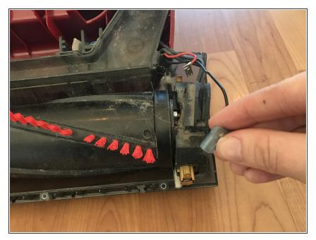
• Remove the negative motor terminal that is located on the bottom right corner of the brush roll.
