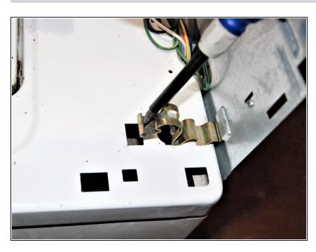
Use the flat head screwdriver to pry out clips on left and right side on top of the machine where the control panel was.
