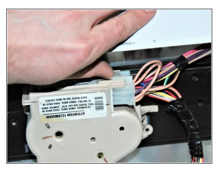
Lift the plastic tab on the timer wiring harness connector and pull from the timer.
