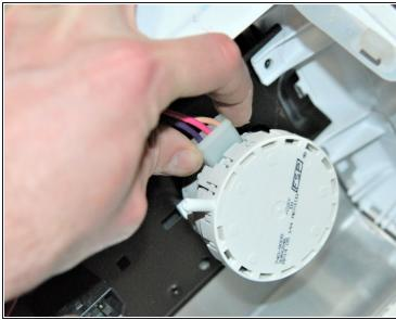
• Disconnect the hose and wiring harness from water level control.
