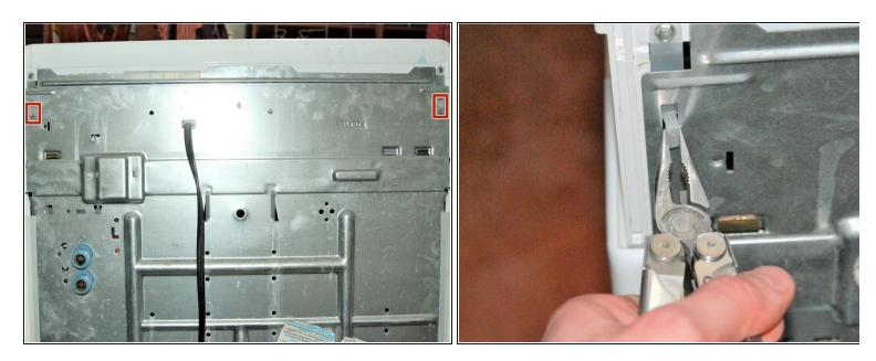
• Pinch the plastic tabs with the needle nose pliers and push through the metal back panel.
