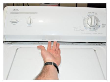
Pull up the control panel located on top of the washer machine.
