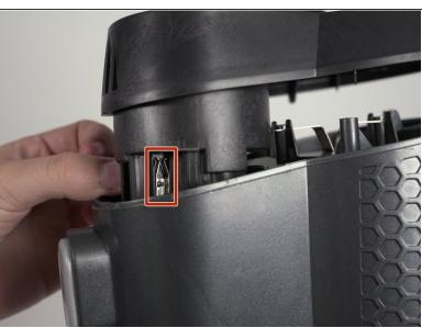
Pry the panel up using a spudger and pull up firmly just enough to see the clips of wire on the sides.
