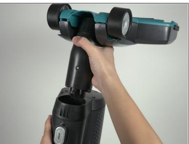
Press the release button while pulling up on the head of the vacuum to remove the head.
