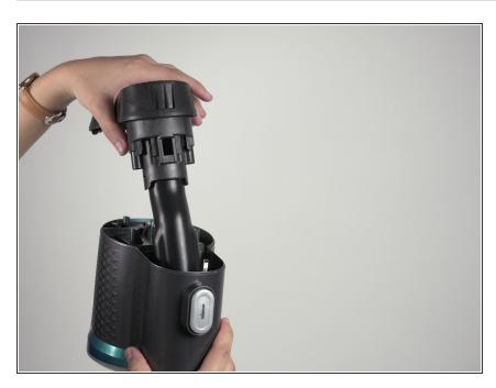
Pull the top piece out of the shaft.
