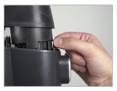
Remove the wire clips on both sides of the shaft.
