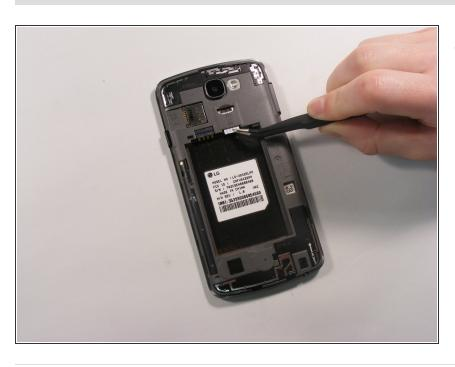
Use Tweezers to pull down on the SIM Card to completely remove.
