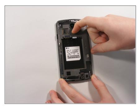
Insert fingernail in groove between SIM card and base of phone, pushing down on the SIM Card to begin removal.
