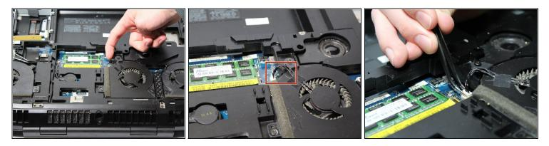
• The fan will be connected to the motherboard by a cable. Use plastic <u>tweezers</u> to gently unplug this connection.
