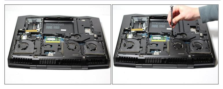
• With the back cover removed, locate the desired fan to replace.
