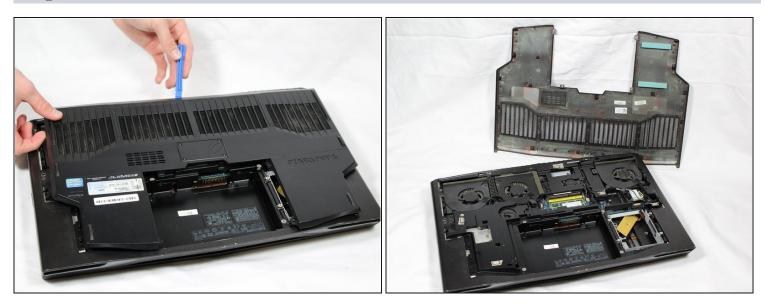
• Use the plastic pryer tool to lift the bottom cover off.
