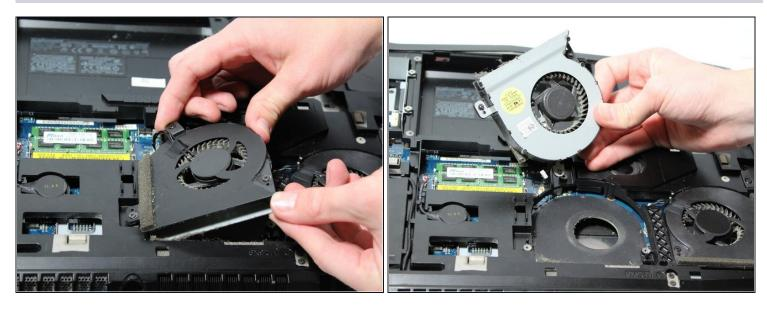
• The fan is now fully disconnected from the computer. Gently remove the fan by lifting upwards.
