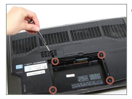
• Unscrew the four indicated screws with a J000 screwdriver.
