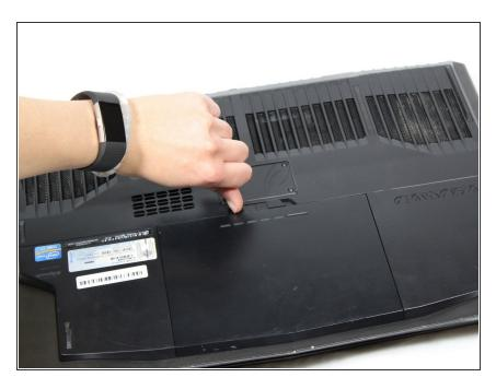
Flip the laptop over and slide the battery release latch to the right.
