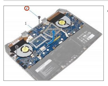
Remove the screws that secure the system board to the computer base.
