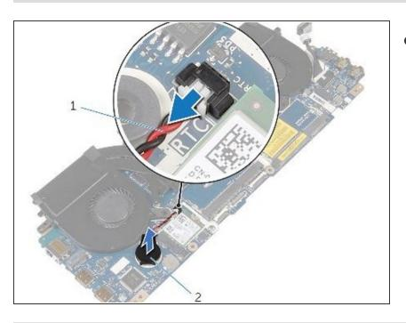
Connect the coin-cell battery cable to the connector on the system board.
