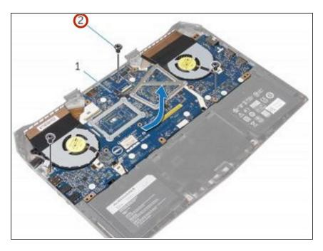
Remove the screws that secure the system board to the computer base.
