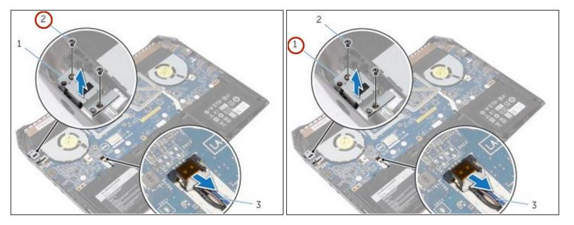
Remove the screw that secures the power-adapter port bracket to the power-adapter port.
