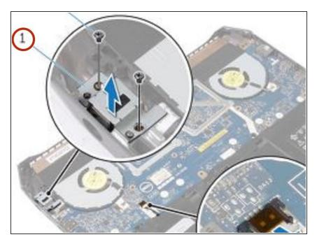
Align the power-adapter port to the computer base.
