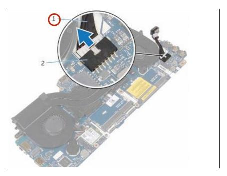
Disconnect the power-adapter port cable and remove the poweradapter port from the system board.
