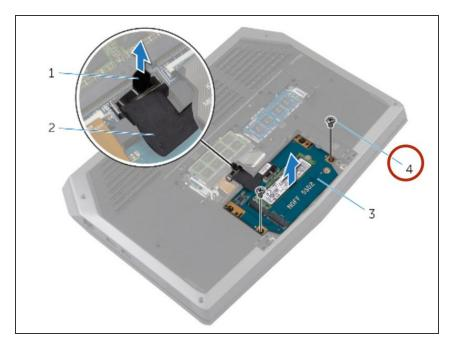
Remove the screws that secure the solid-state drive assembly to the computer base.
