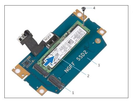
Slide and lift the solid-state drive off the solid-state assembly.
