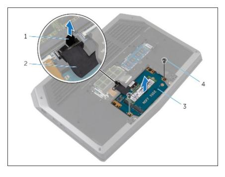
Replace the screws that secure the solid-state drive bracket to the solidstate drive assembly.
