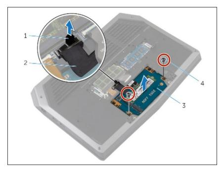
Replace the screw that secures the solid-state drive assembly with the screw holes on the computer base.
