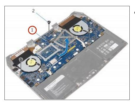
Slide and lift the system-board assembly.
