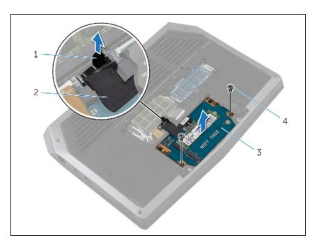
Connect the solid-state drive cable to the system board.
