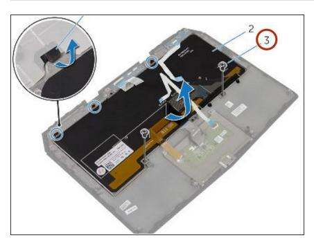
Align the screw holes on the NEW keyboard with the screw holes on the palm-rest assembly.
