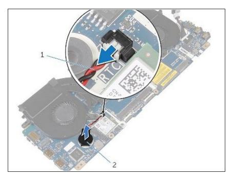
Adhere the **NEW** coin-cell battery to the system board.
