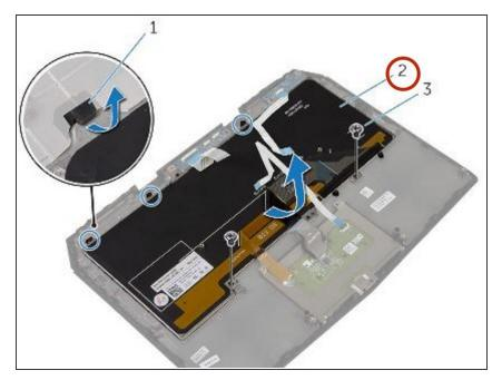
Slide and lift the keyboard, along with the cables, off the palm-rest assembly.
