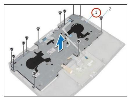
Lift the keyboard bracket off the palm-rest assembly.
