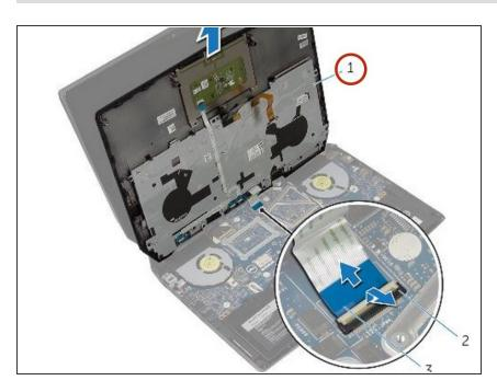
Align the palm-rest assembly on the computer base and snap it into place.
