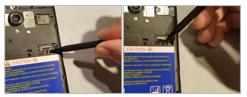
Disconnect the battery connector flex cable by sliding the black spudger under the wires and carefully prying up the entire terminal casing.
